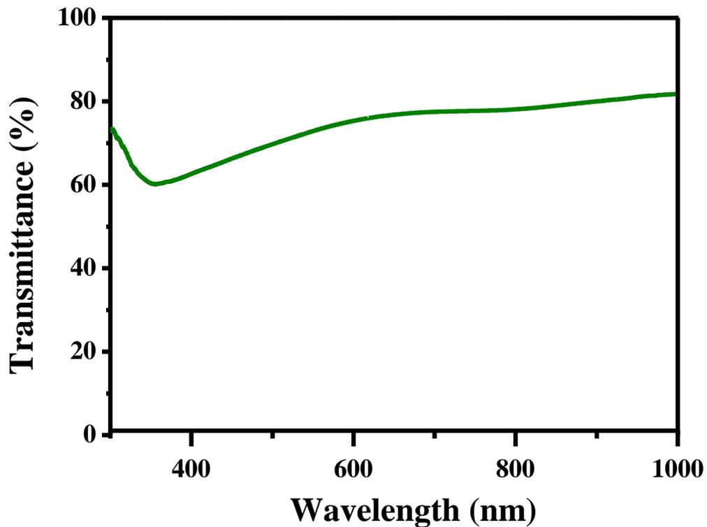
Figure 3: Optical absorbance and transmittance spectrum of spray deposited MoS<sub>2</sub> thin film
