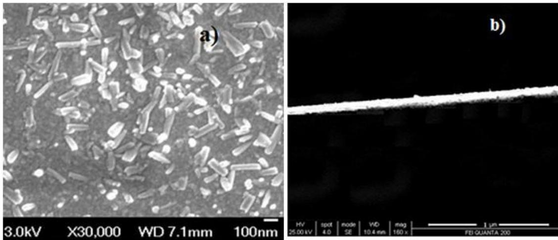
Figure 2: (a) FE-SEM and (b) Cross-sectional SEM of MoS<sub>2</sub> thin film
