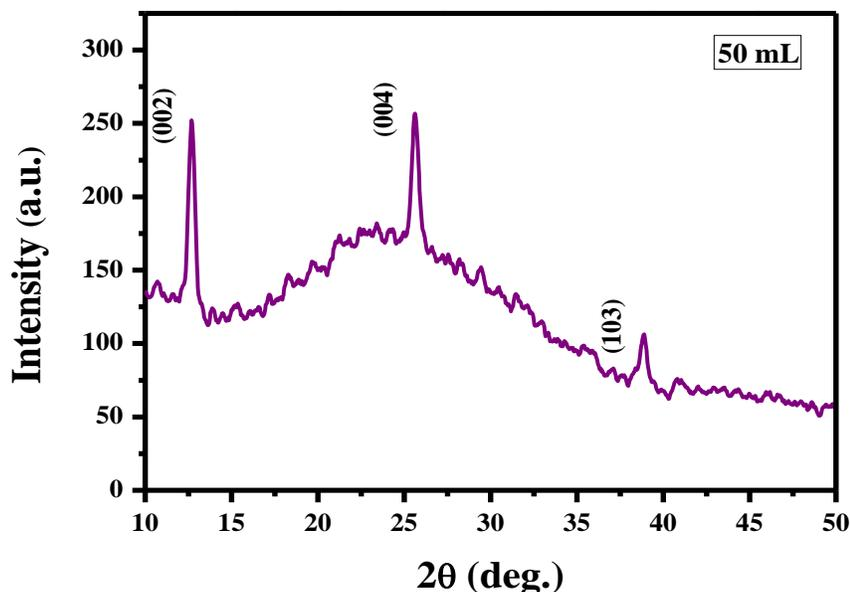
Figure 1: Structural morphology of 50 mL deposited MoS<sub>2</sub> thin film
